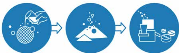
Figure 1: (i) Via capillary forces, an oily API is readily adsorbed onto the Fujisil in order to create (ii) the free-flowing oil-loaded powder, prior to the tableting process to create (iii) Hard tablets without oil leakage.
